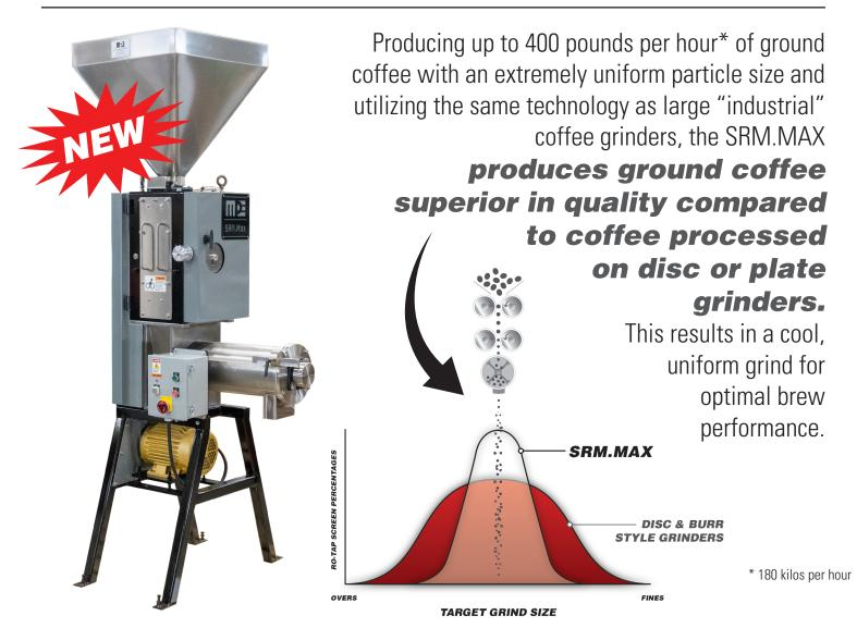
The Superior Quality of a Roller-Style Grinder at the Size and Cost of an Industrial Sized Disc Grinder
